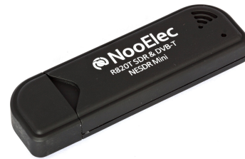
Fig. 3. RTL2832U SDR with a Raphael R820T tuner.
