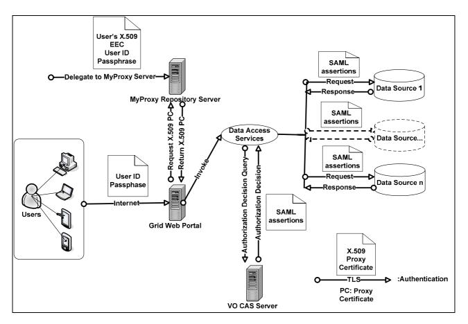
Figure 3. Generalised Security Architecture
